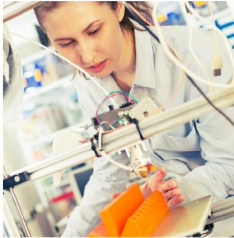
3D printers are able to create a three-dimensional object by applying layers of material following a computer's instruction. The process of 3D printing is also called additive manufacturing, because the printed object is created by adding layer upon layer of material. The printing material can be anything from plastics to human cells to sugar.
